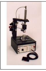
**Process: Nondestructive, Fast, Clean** Permanent inscriptions are made in seconds. Mild electrolyte and low voltage current etch the metal surface through openings in a stencil. Only the legend in the stencil is etched into the part surface. Marks/inscriptions cover from very small to large areas. Depth, darkness and shade of inscription are controlled through time, current, electrolyte and marking cycle.
